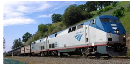
Figure 1: P-42 Diesel locomotive hauling a long distance train
