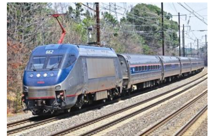
Figure 11: HHP-8 electric locomotive
