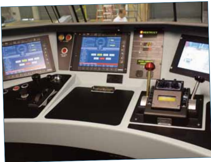
Powering Up: Plans to add 70 electric locomotives – currently on order from Siemens – took a major step forward. The first ACS-64 electric engine is scheduled to be delivered in fiscal year 2013 and will operate at speeds of up to 125 mph. Engineers tested this mock-up of the cab at the Siemens manufacturing facility in Sacramento, CA.
