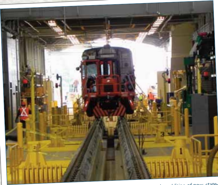
Modern Facilities: Los Angeles and Hialeah, FL (shown here), saw the addition of new, state-of-the-art maintenance facilities, and Seattle's facility is currently under construction. The facilities are designed using a "progressive spot" approach, meaning the cars move through a standard production line in a way that maximizes efficiency.
