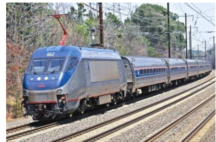
Figure 11: HHP-8 electric locomotive
