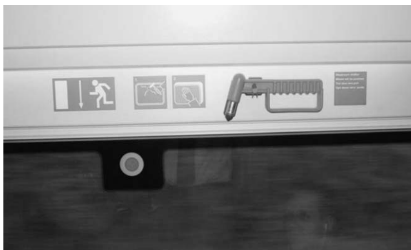
Actual emergency device in the interior compartment of the DB high-speed ICE train.
