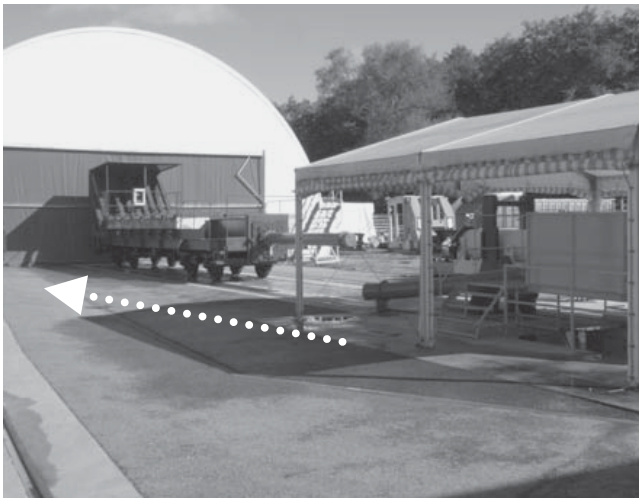
Tests are conducted on actual rail cars and locomotives. A gas-fired rail car is propelled at high speeds into locomotive and car ends that employ various types of crash buffers.
