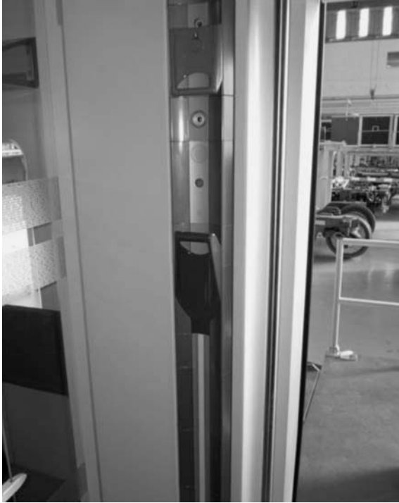
Emergency door controls and an intercom button aboard a new rail vehicle.
