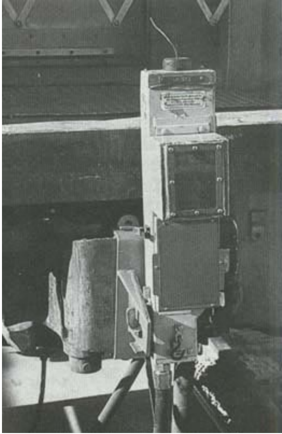
Photo 3: E.O.T. mounted on knuckle mount bracket
