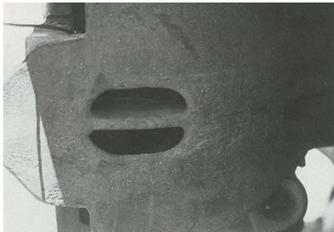
Photo 6: Coupler draft holes
